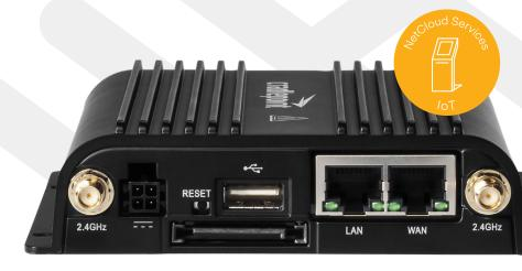
Cradlepoint IBR600C Series IoT routers are semi-ruggedized, cloud-managed LTE routers, built for IoT, M2M, and Work from Anywhere applications. They provide a resilent, LTE connection ideal for use in high-availability, portable, or fixed uses. The IBR600C Series is available with either IoT or SOHO NetCloud Service Plans, which provide features optimized for each unique deployment.
